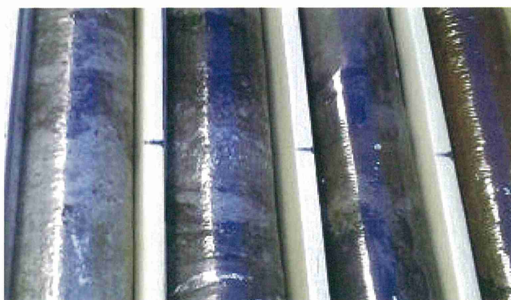
“泥岩・粘土・凝灰質”互層掘削
